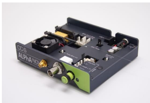
Figure 10 : Alphanov SOA driver able to modulate light down to 1ns with very high extinction ratio of more than 50dB.
