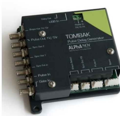
Figure 2 : Example of fast switching synchronization electronics from Alphanov
