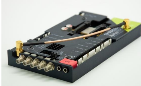
Figure 7 : Shaper board for EOM driving, combining a laser diode driver, a multiple output synchronization electronics and a 5V programmable shape output to drive an EOM with 2GHz bandwidth and 48dB dynamic range
