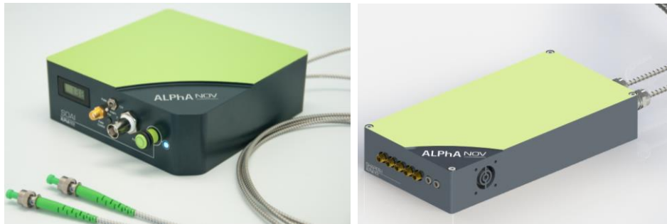
Figure 11 : Turn-key SOM with several interesting functionalities and USB control. Square shape version (left) : The pulse width can be adjusted internally or triggered externally with a LVTTTL signal. The peak power is adjusted internally with up to 60dB resolution or externally with a pure analog 0-5V signal. Shaped version with internal AWG (right) ; the shape of the output pulse can be configured with 2GHz bandwidth and 48dB dynamic range.
