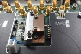
Exemple of butterfly (top) and TOSA (bottom) laser diode
